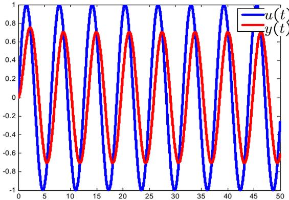
At steady-state,  $u(t)$  and  $y(t)$  has same frequency, but different amplitude and phase!
